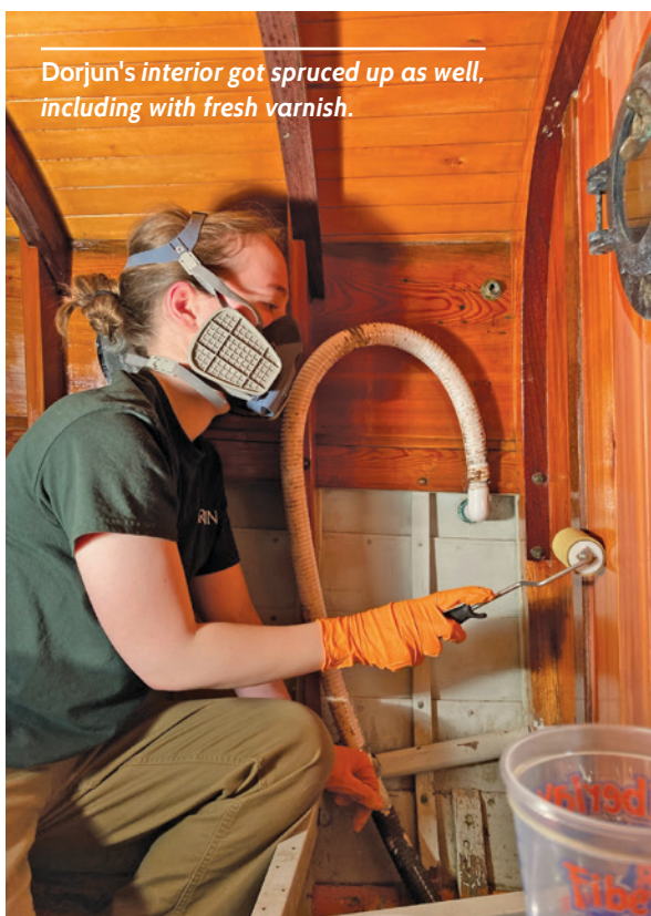
Scraping the bilge to bare wood before installing 74 new rivets to keep water out.
