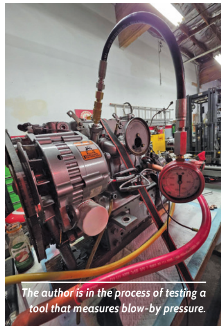
Excessive smoke during normal operation can be a sign of blow-by.
