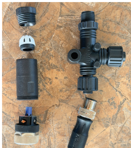
NMEA 2000 spare components: Left is the components of a field installable NMEA 2000 end. Right—tee, terminator.
